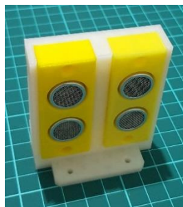
Figure 7-a. Two transmitters having the same transmitting direction
