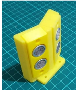
Figure 8-a Two transmitters configured with +/- 18 degrees transmitting angles.
