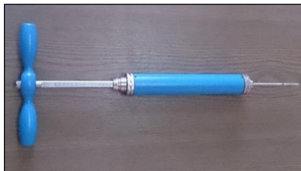
Figure 3. The penetration resistance test apparatus
