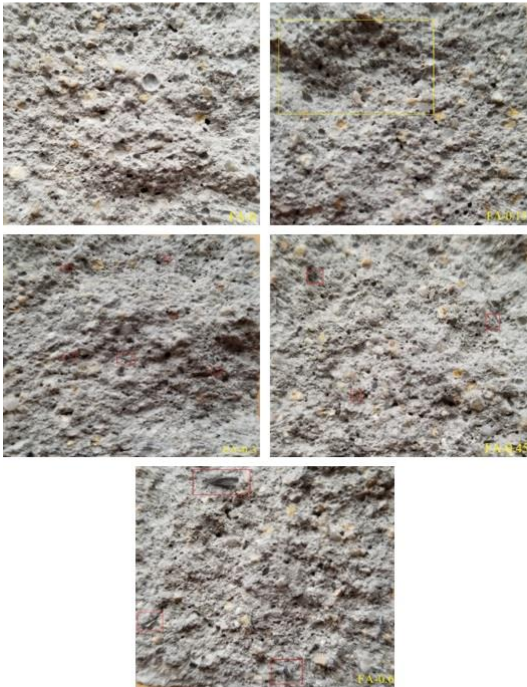
Fig.4. Cross-section fracture images of hybrid FA mortar specimens.
