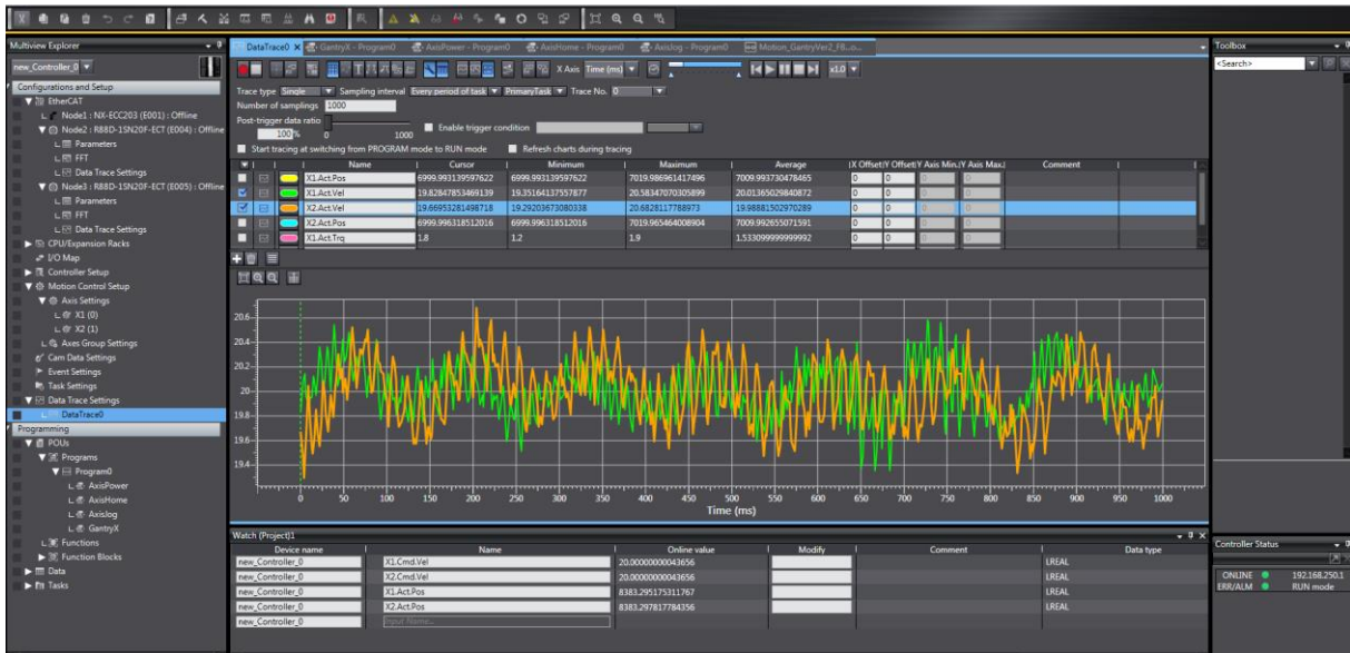
Figure 5. Velocity Values Belonging to Axes After Auto-tuning Process
